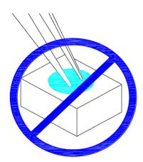
Do not stack together assembled PCBs containing LEDs.
