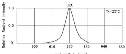
wavelength  $\lambda$  (nm) RELATIVE INTENSITY Vs. WAVELENGTH
