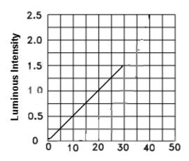
Luminous Intensity Vs. Forward current
