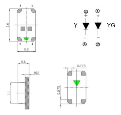
**Note:** Tolerance unless mentioned is  $\pm 0.1$ mm, Unit = mm.
