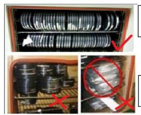
Correct way: material desiccant need to remove the bag, use the way of hanging baked
