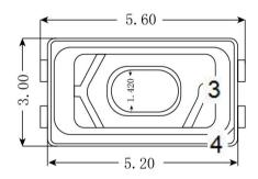
Recommended Soldering Pattern: (Units: mm)
