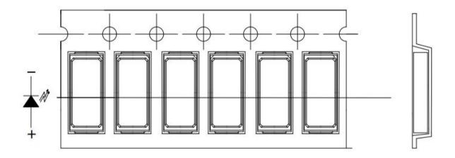
All dimensions in mm, tolerances unless mentioned is ±0.1 mm.
