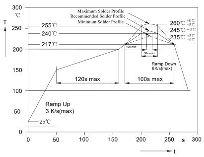
**Remark:** If not lead free soldering, the recommended solder profile is 230°C and max solder profile is 245°C.
