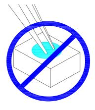
2. The outer diameter of the SMD pickup nozzle should not exceed the size
