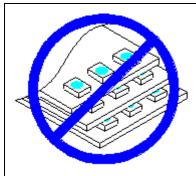
5.LED operating environment and sulfur element composition cannot be over 100PPM in the LED mating usage material.
