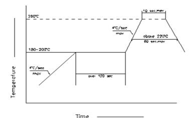
1.Reflow soldering should not be done more than two times.
