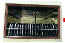
Correct way: material desiccant need to remove the bag, use the way of hanging baked
