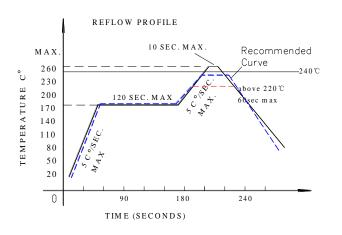
Reflow soldering should not be done more than three times.
