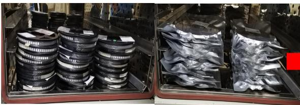
Wrong way: the material is dehumidified without removing the bag, in a stacking manner
