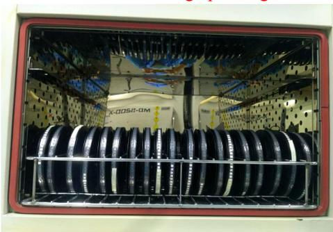
Correct way: material desiccant need to remove the bag, use the way of hanging baked
