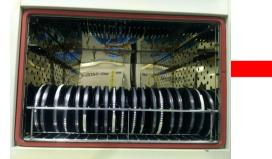
Correct way: material desiccant need to remove the bag, use the way of hanging baked
