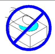
2.The outer diameter of the SMD pickup nozzle should not exceed the size of the LED to prevent air leaks. The inner diameter of the nozzle should be as large as possible. A pliable material is suggested for the nozzle tip to avoid scratching or damaging the LED surface during pickup. The dimensions of the component must be accurately programmed in the pick-and-place machine to insure precise pickup and avoid damage during production.
