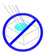
2. The outer diameter of the SMD pickup nozzle should not exceed the size of the LED to prevent air leaks. The inner diameter of the nozzle should be as large as possible. A pliable material is suggested for the nozzle tip to avoid scratching or damaging the LED surface during pickup. The dimensions of the component must be accurately programmed in the pick-and-place machine to insure precise pickup and avoid damage during production.
