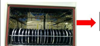
Correct way: material desiccant need to remove the bag, use the way of hanging baked
