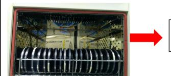
Correct way: material desiccant need to remove the bag, use the way of hanging baked
