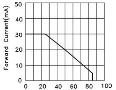
FORWARD CURRENT DERATING CURVE
