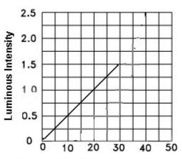
Luminous Intensity Vs. Forward current
