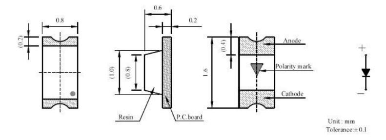
**Note:** Tolerance unless mentioned is  $\pm 0.1$ mm,Unit = mm.
