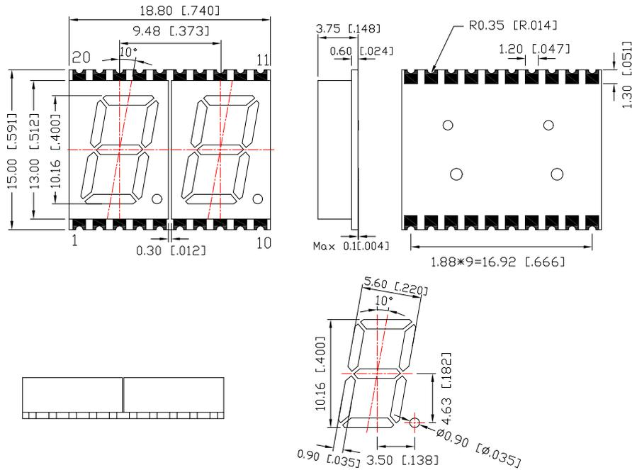
Tolerance is  $\pm 0.25\text{mm}$  unless otherwise noted, Unit=mm
