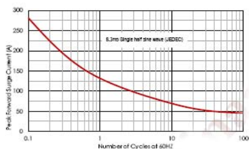
Fig 3 Maximum Non-Repetitive Forward Surge Current
