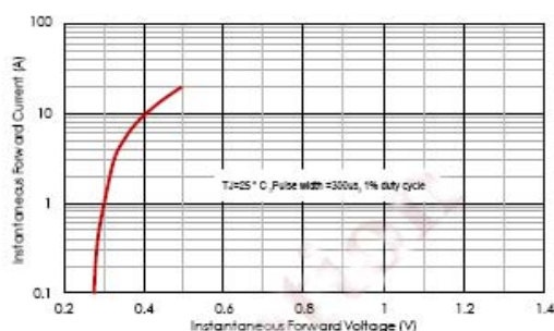
Fig 2 Typical Instantaneous Forward Characteristics
