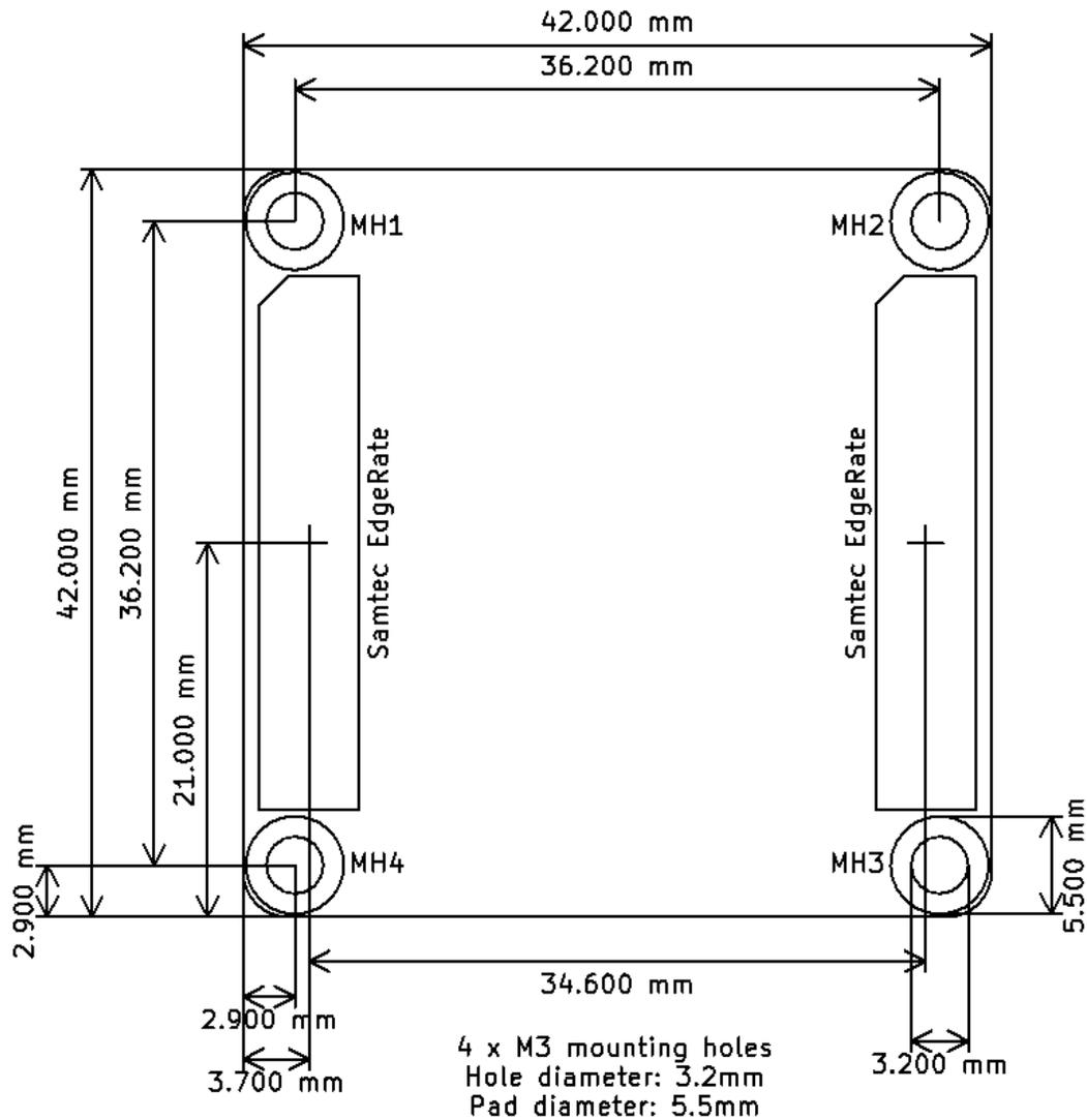
Figure 9. UbiSwitch mechanical drawing, viewed from top down
