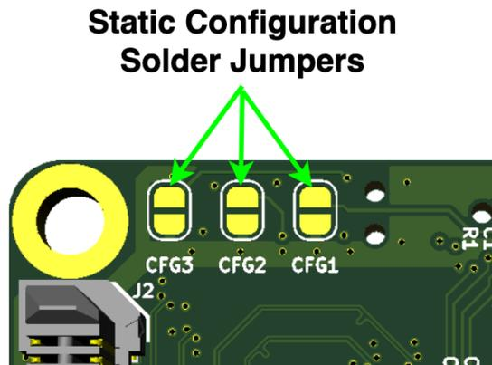
Figure 7 - The static configuration headers on UbiSwitch
