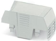
DIN rail housing, Upper housing part, flat design, connection opening on one side, connection opening on one side, width: 35.1 mm, height: 74.65 mm, depth: 36.95 mm, color: light gray (similar RAL 7035)
