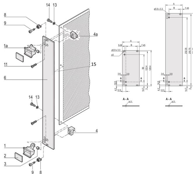
Plug-in unit, with extraction handle type 1 and flat panel. The grey handle is assembled on the front panel.
