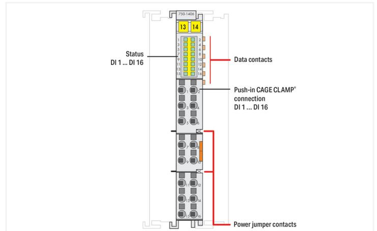
This digital input module features 16 channels in a width of just 12 mm (0.47 inch). The module features Push-in CAGE CLAMP® connections enabling solid conductors to be connected by simply pushing them in. Each input channel has a noise-rejection RC filter with 0.2 ms time constant. A green LED indicates the signal state of each channel. Field and system levels are electrically isolated. An operating tool with a 2.5 mm blade (210-719) is required to open the Push-in CAGE CLAMP® connections.
