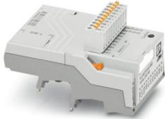
PLC logic basic module, Generation 2, with 16 I/Os, for plug-in connection to eight digital or analog PLC-INTERFACE terminal blocks, can be extended to 48 I/Os, real-time clock, micro USB female connector, accommodates memory module and Bluetooth adapter, Push-in connection
