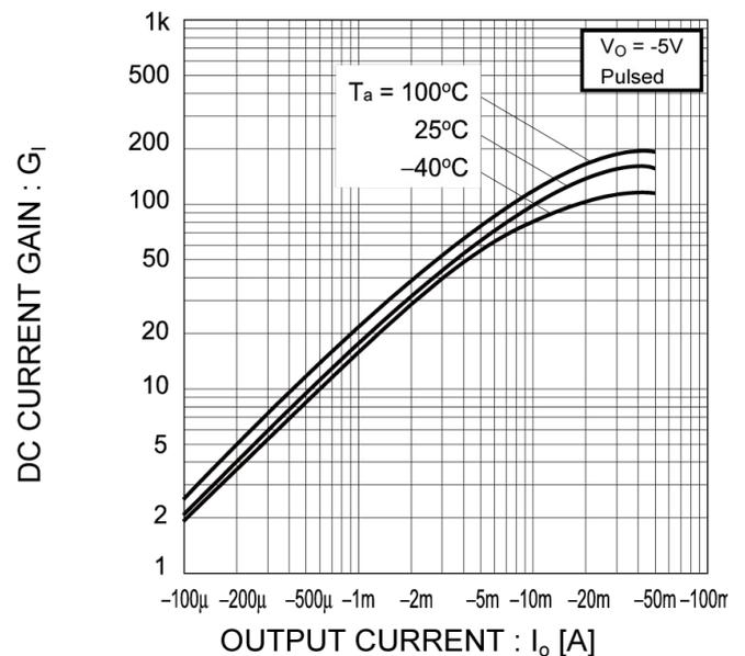
● Electrical characteristic curves ( $T_a=25^\circ\text{C}$ ) <For DTr2(PNP)>
