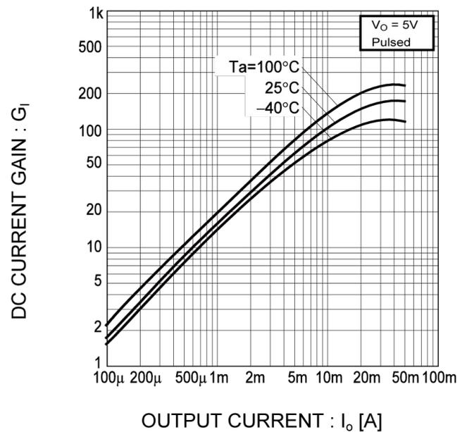
● Electrical characteristic curves ( $T_a = 25^\circ\text{C}$ ) <For DTR1(NPN)>
