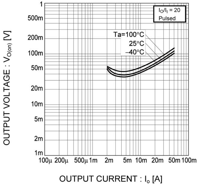
●Electrical characteristic curves( $T_a=25^{\circ}\text{C}$ ) <For DTr2(PNP)>
