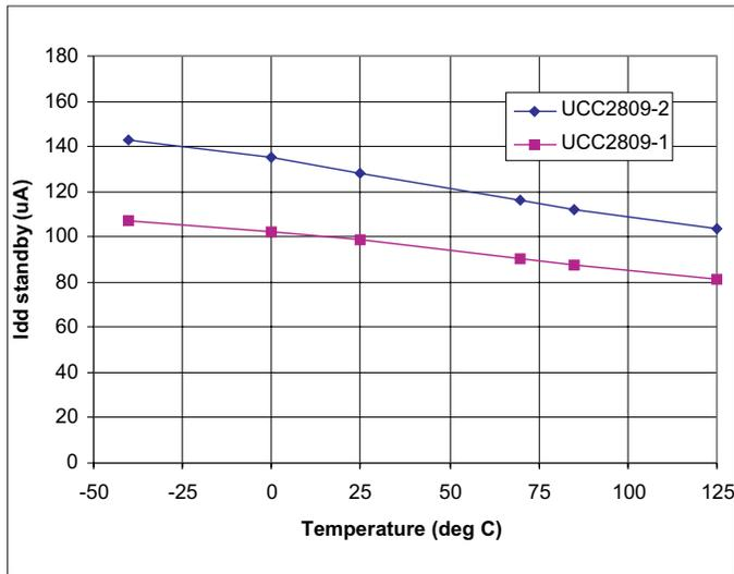
Figure 6. I<sub>DD</sub> (standby) vs. temperature.
