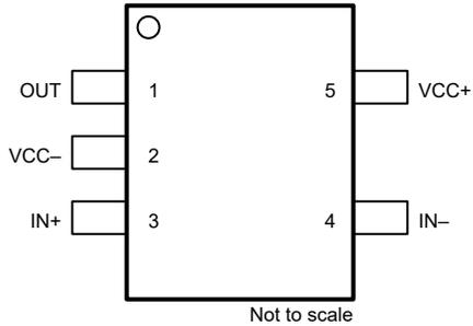
**Figure 4-1. TL071H DBV Package, 5-Pin SOT-23 (Top View)**
