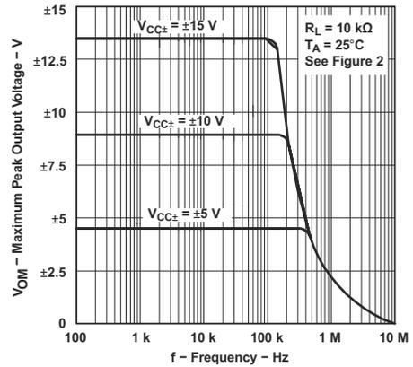
Figure 5-39. Maximum Peak Output Voltage vs Frequency
