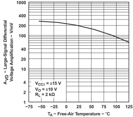
**Figure 5-45. Large-Signal Differential Voltage Amplification vs Free-Air Temperature**
