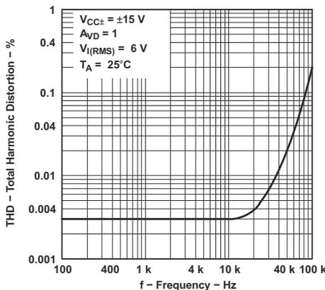
Figure 5-54. Total Harmonic Distortion vs Frequency
