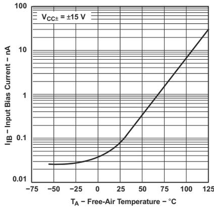
Figure 5-38. Input Bias Current vs Free-Air Temperature
