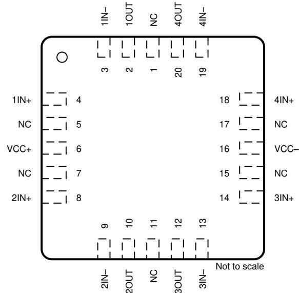
**Figure 4-9. TL074M FK Package, 20-Pin LCCC (Top View)**
