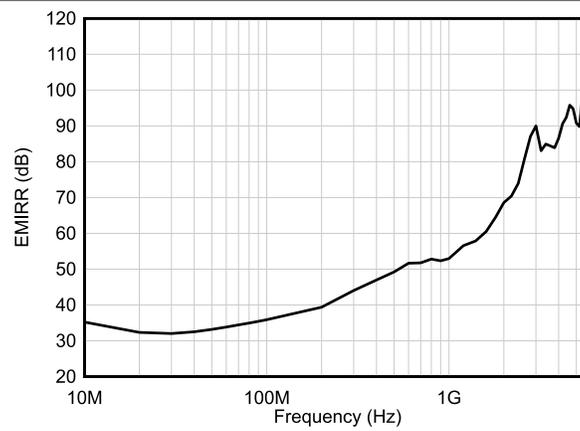
Figure 5-37. EMIRR (Electromagnetic Interference Rejection Ratio) vs Frequency
