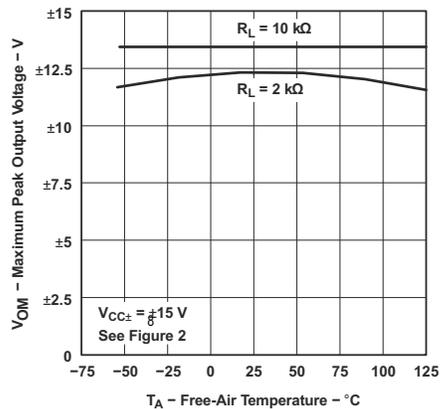
Figure 5-42. Maximum Peak Output Voltage vs Free-Air Temperature
