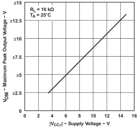
**Figure 5-44. Maximum Peak Output Voltage vs Supply Voltage**
