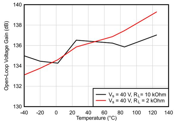
Figure 5-21. Open-Loop Voltage Gain vs Temperature
