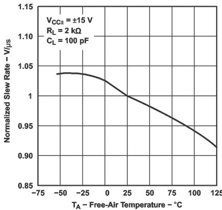
Figure 5-52. Normalized Slew Rate vs Free-Air Temperature
