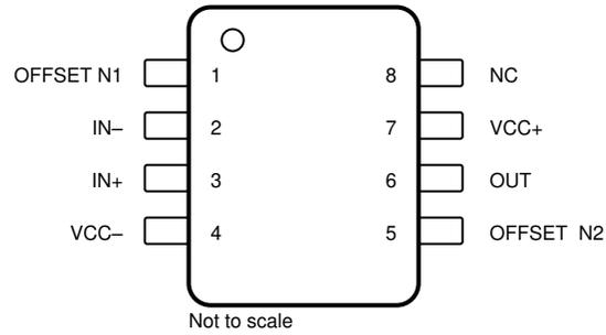
**Figure 4-4. TL071C PS Package, 8-Pin SO
