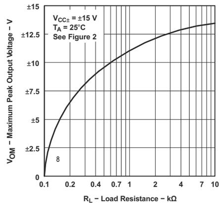
Figure 5-43. Maximum Peak Output Voltage vs Load Resistance
