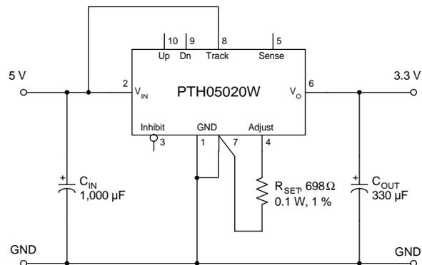
When the *Track* pin is connected to the input voltage the Auto-Track function is permanently disengaged. This allows the module to power up entirely under the control of its internal soft-start circuitry. When power up is under soft-start control, the output voltage rises to the set-point at a quicker and more linear rate.
