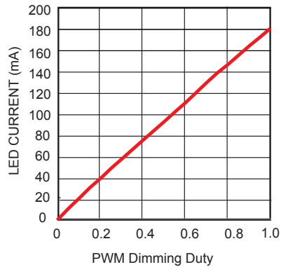
LED Current vs. PWM Dimming Duty
