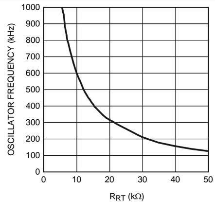
Figure 4. Frequency vs  $R_T$
