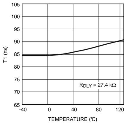
Figure 9. SR T1 Parameter vs Temperature
