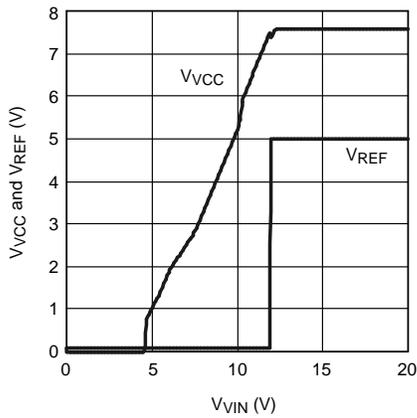
Figure 1.  $V_{CC}$  and  $V_{REF}$  vs  $V_{IN}$
