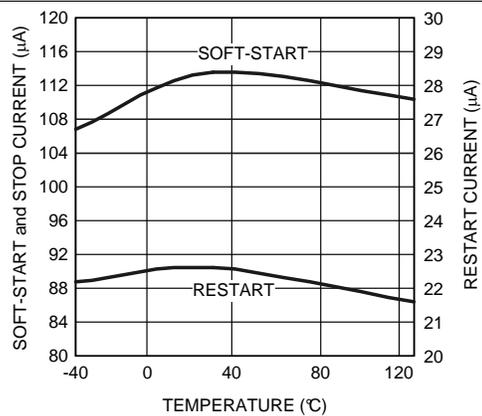
Figure 6. Soft-Start Current vs Temperature
