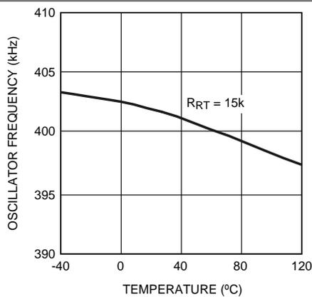
Figure 5. Oscillator Frequency vs Temperature
