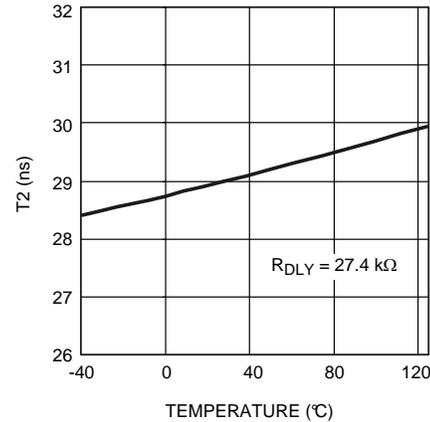
Figure 10. SR T2 Parameter vs Temperature
