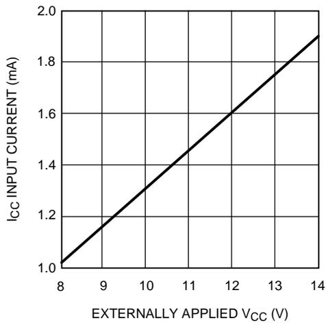
Figure 1. I<sub>CC</sub> Current vs Applied V<sub>CC</sub> Voltage
