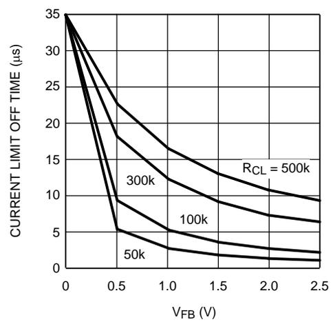
Figure 4. Current Limit Off-Time vs V<sub>FB</sub> and R<sub>CL</sub>
