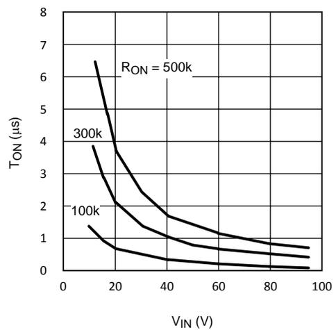
Figure 2. On-Time vs Input Voltage and R<sub>ON</sub>
