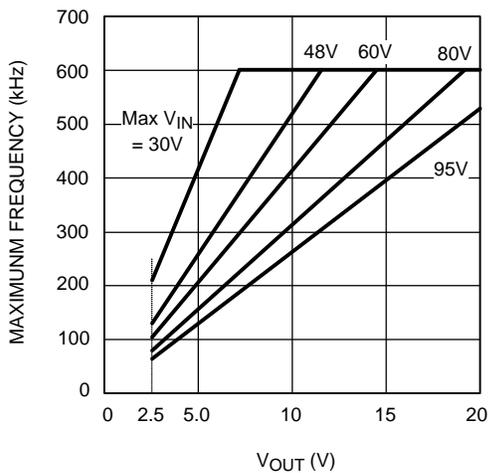
Figure 3. Maximum Frequency vs V<sub>OUT</sub> and V<sub>IN</sub>
