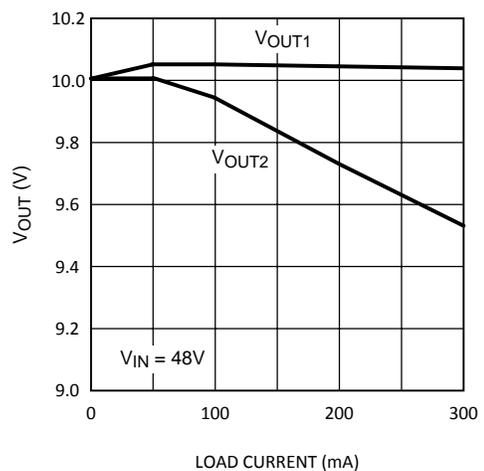
Figure 6. Output Voltage vs Load Current
