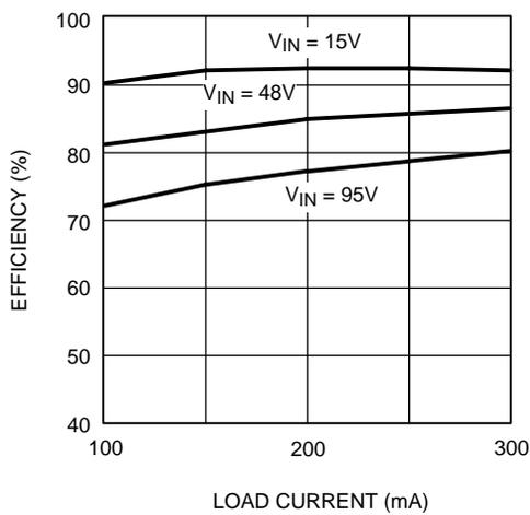
Figure 5. Efficiency vs Load Current vs V<sub>IN</sub>
