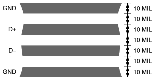
Figure 19. Arrangement of Signal Tracks
