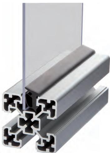
**Assembly:** Insert the panel into the profile slot. Then press the profile seal into the slot by hand or using a blunt object.
