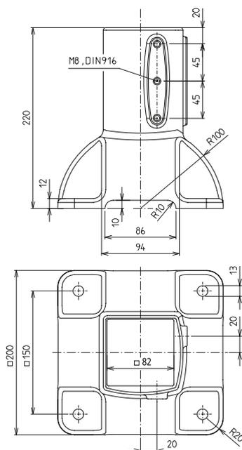
**Material:** Silver powder-coated gravity die-cast aluminium, stainless steel fixing
