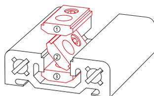
Example of retrospective insertion of an N slot stone in a profile.
