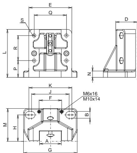
Clamping using slot stone -L-
