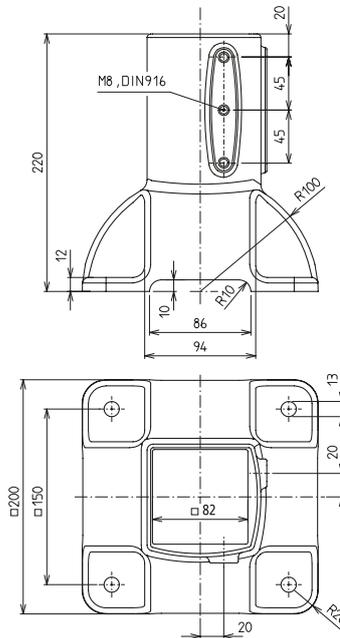
**Material:** Silver powder-coated gravity die-cast aluminium, stainless steel fixing
