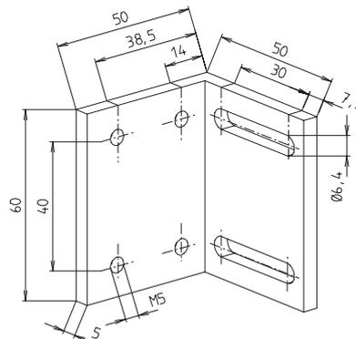
Fixing set for lifting door
