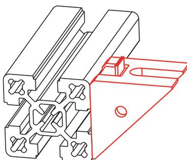
**Angle bracket perpendicular to the profile:**
