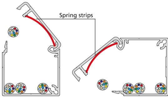
Assembly strips facilitate overhead assembly
