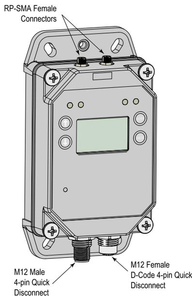
**Connectivity**—The DXM1200-B2's wired and wireless connectivity options make it easy to share data between local and remote equipment. The cellular modem option eliminates the need for IT infrastructures to connect remote equipment for sensing and control to IIoT cloud services. The integrated Sure Cross® wireless radio enables Modbus connectivity to remote sensors, indicators, and control equipment.
