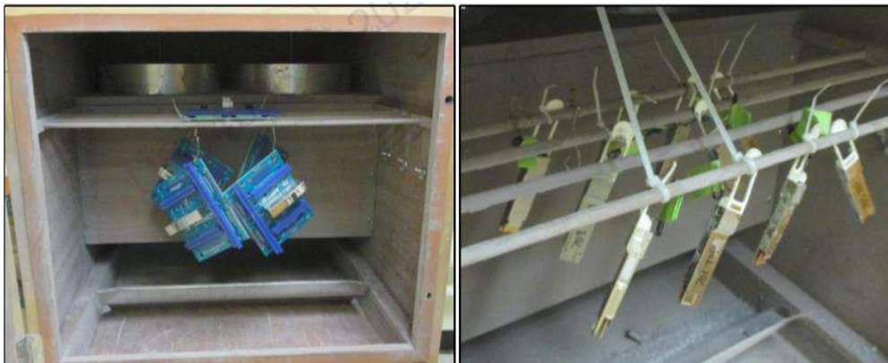
Figure 5 - Typical Benign Dust Contamination Test Setup
