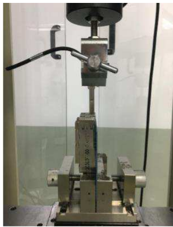
Test setup (mating force)
