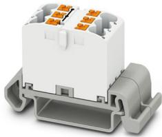
Distribution block, Block with horizontal alignment, nom. voltage: 690 V, nominal current: 24 A, number of connections: 6, connection method: Push-in connection, cross section: 0.14 mm<sup>2</sup> - 4 mm<sup>2</sup>, mounting type: NS 35/7,5, NS 35/15, color: white
