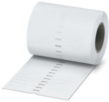
Marker strip, Roll, white, unmarked, can be labeled with: THERMOMARK E.300 (D)/600 (D), THERMOMARK ROLL 2.0, THERMOMARK ROLL, THERMOMARK ROLL X1, THERMOMARK ROLLMASTER 300/600, THERMOMARK X1.2, mounting type: adhesive, Number of individual labels: 2500, text field height: 2.8 mm, text field width: 104 mm
