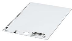
Marker for terminal blocks, Card, white, unmarked, can be labeled with: BLUEMARK ID COLOR, BLUEMARK ID, THERMOMARK PRIME, THERMOMARK CARD 2.0, THERMOMARK CARD, THERMOMARK PRIME 2.0, mounting type: adhesive, Number of individual labels: 26, text field height: 2.8 mm, text field width: 104 mm
