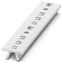
Zack marker strip, Strip, white, labeled, horizontal: L1, L2, L3, N, PE, L1, L2, L3, N, PE, mounting type: latching, for terminal block width: 5.2 mm, Number of individual labels: 10, text field height: 10.5 mm, text field width: 5.15 mm
