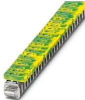
Connection terminal block, nom. voltage: 300 V, nominal current: 41 A, connection method: Screw connection, Rated cross section: 4 mm<sup>2</sup>, cross section: 0.5 mm<sup>2</sup> - 6 mm<sup>2</sup>, mounting: Neutral busbar, color: green-yellow
