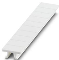
Zack marker strip, Strip, white, unmarked, can be labeled with: PLOTMARK, CMS-P1-PLOTTER, mounting type: latching, for terminal block width: 5.2 mm, Number of individual labels: 10, text field height: 10.5 mm, text field width: 5.1 mm
