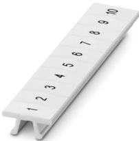
Zack marker strip, Strip, white, labeled, printed horizontally: consecutive numbers 1 ... 10, 11 ... 20, etc. up to 491 ... 500, mounting type: latching, for terminal block width: 5.2 mm, Number of individual labels: 10, text field height: 10.5 mm, text field width: 5.15 mm
