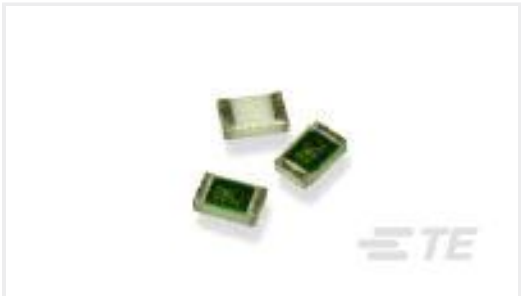
TE Part #5-1879216-1 CPF0402 255K 0.1% 25PPM 1K RL
