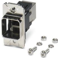
RJ45 panel mounting frame, IP67, for push-pull interlocking, metal, for rectangular mounting cutout, with seal and mounting screws, incl. RJ45 coupling module
