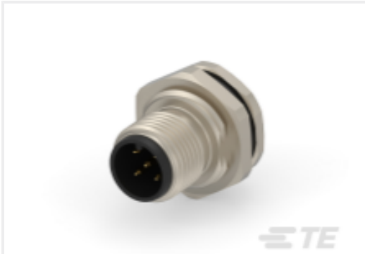
TE Part #T4171010005-001 M12,REAR MOUNTING,MALE,A,5P,0.2 M WIRE
