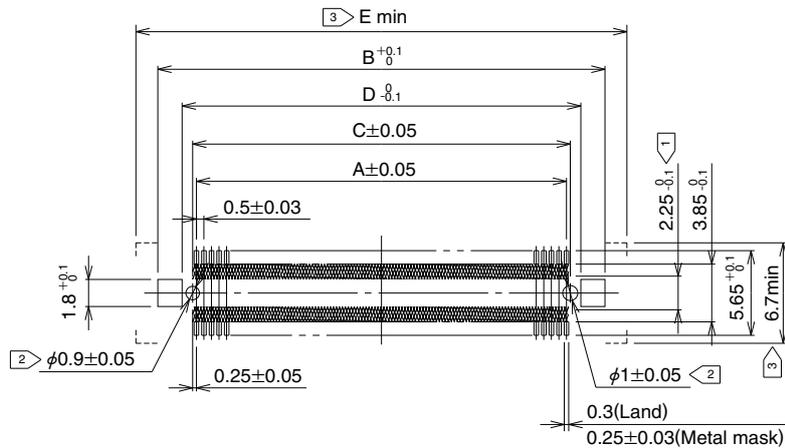
Note ① The cross-hatched area inside the SMT land may come into contact with the connector contacts and thus care should be taken that the pattern does not extend beyond the SMT land width.
