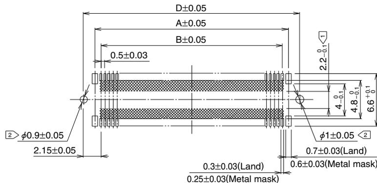
Note ① The cross-hatched area inside the SMT land may come into contact with the connector contacts and thus care should be taken that the pattern does not extend beyond the SMT land width.
