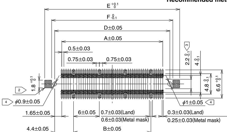
Note ① Cross-hatched portions, totaling n places, indicate the ground circuits.
