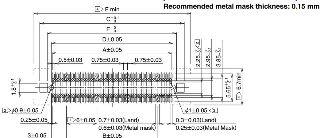
Note ① Cross-hatched portions, totaling n places, indicate the ground circuits.
