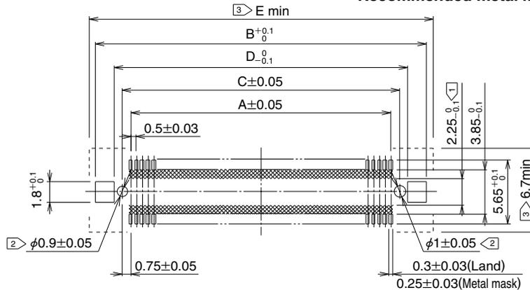
Note ① The cross-hatched area inside the SMT land may come into contact with the connector contacts and thus care should be taken that the pattern does not extend beyond the SMT land width.
