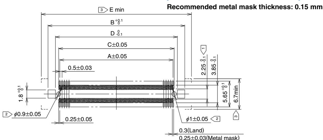
Note ① The cross-hatched area inside the SMT land may come into contact with the connector contacts and thus care should be taken that the pattern does not extend beyond the SMT land width.
