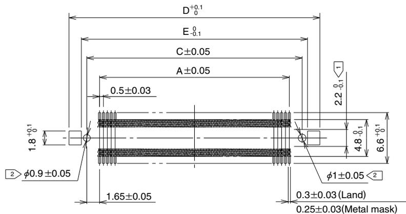
Note ① The cross-hatched area inside the SMT land may come into contact with the connector contacts and thus care should be taken that the pattern does not extend beyond the SMT land width.
