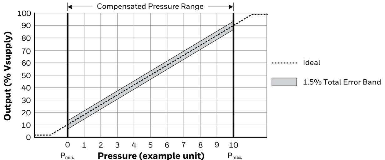
$$\text{Output (V)} = \frac{0.8 \times V_{\text{supply}}}{P_{\text{max.}} - P_{\text{min.}}} \times (\text{Pressure}_{\text{applied}} - P_{\text{min.}}) + 0.10 \times V_{\text{supply}}$$
