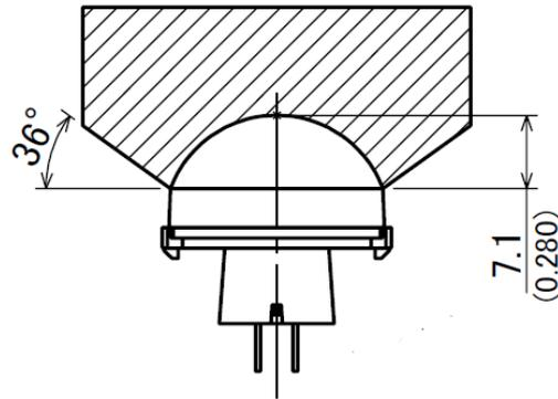
Recommended Hole Drilling Diameter
