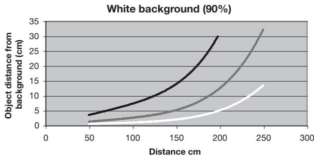
In this mode the maximum operating frequency is set to 250 Hz and detection is optimized for objects close to the background for top performance in general industry automation applications such as pallet wrapping machines, airport baggage conveyors, wood planks handling/stacking.
