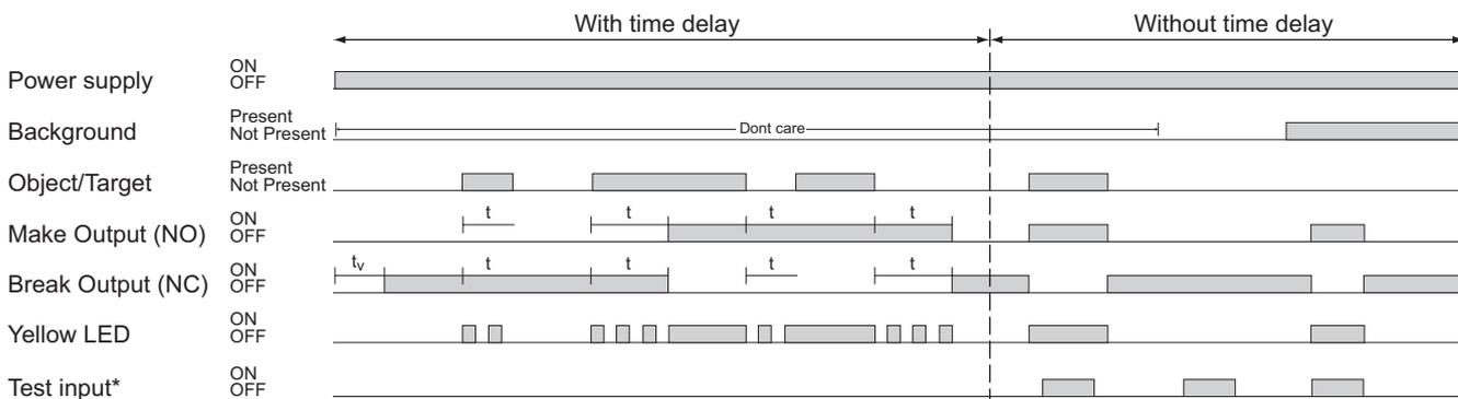
t<sub>v</sub> = Power on delay, t = Time delay (delay on operate and delay on release)
